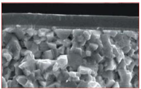
Figure N°1- DLC coating on sintered carbide (Korloy – Corea)
