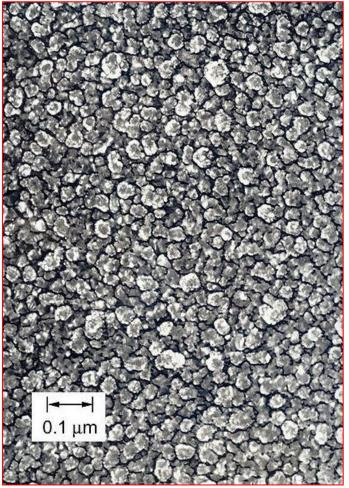
Figure N°2- Crystals of C present in a layer of DLC
