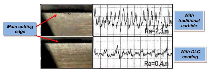
Figure N°4- Example of reduction of surface roughness using DLC coatings
